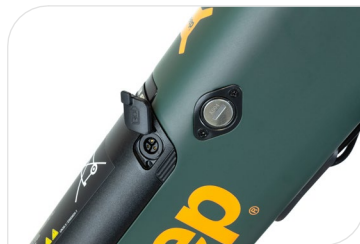
36 V, 13.5 Ah, 650 Wh Greenway battery, smart BMS
